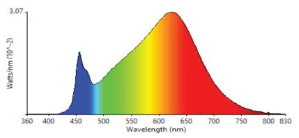
Testing was performed in accordance with LM-79-08.
